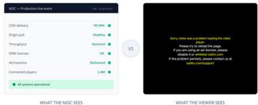
Figure 1. Same break, same moment. The NOC reports every system healthy across CDN, origin, DRM and ad insertion. On the device, the ad break has failed. Resilience depends on watching both views, because only one matches the viewer's experience.
