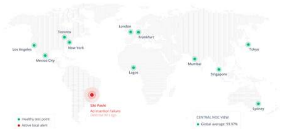
Figure 2. Distributed test devices across viewer regions. The central NOC reads a healthy 99.97% global average; the São Paulo robot has detected a local ad insertion failure that the global metric smooths out. The fix can be pushed before the regional viewer experience degrades.
